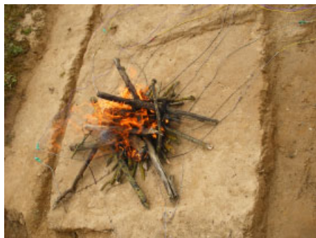
Figure 16. Real fire used to heat the soil.
