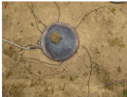
Figure 11. Electrical plate is put on the soil.
