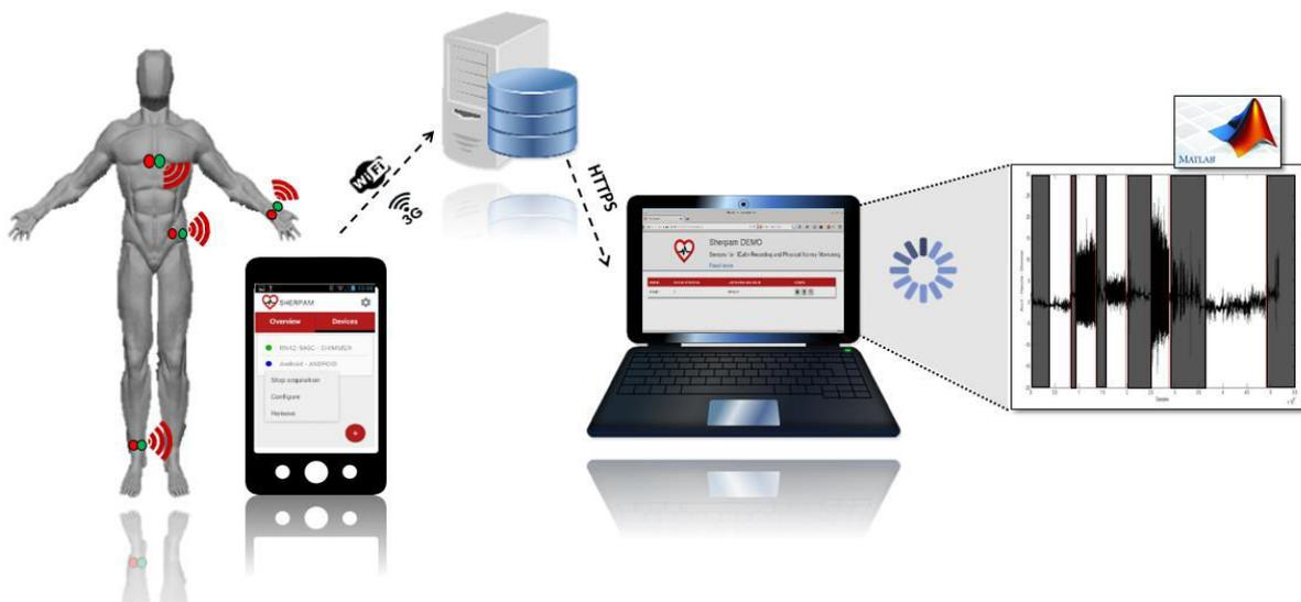
Figure 1.1 - The chain of collecting, transmitting and processing data in SHERPAM project.
