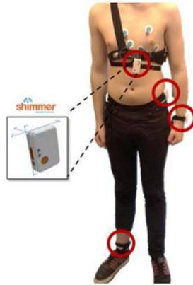
Figure 3.1 - The Shimmer sensor nodes and the ECG electrodes positions on the body in the basic protocol.
