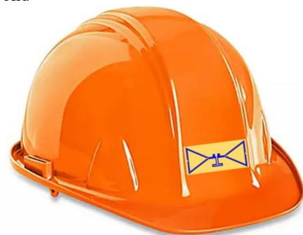
Fig. 1. A safety helmet equipped with the proposed RFID tag.
