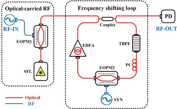
Fig. 1. Experimental set-up. See text for details.
