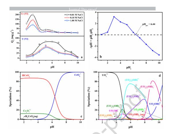
Figure 3. The effect of different pH and ionic strength on the adsorption of Cr(VI) and U(VI) onto CS-TFT (a). [CS-TFT] = 0.2 g L<sup>-1</sup>, [Cr(VI)] = 100 mg L<sup>-1</sup> or [U(VI)] = 20 mg L<sup>-1</sup>; T= 308K; The Zeta potential of CS-TFT (b). The speciation of 100 mg L<sup>-1</sup> Cr(VI) and 20 mg L<sup>-1</sup> U(VI) as a function of pH with 0.01 M ionic strength was obtained by the Visual MINTEQ program (c and d).
