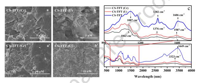
**Figure 6**. SEM images CS-TFT after adsorption of (a and a') Cr(VI) and (b and b') U(VI). (c) FTIR spectra of CS-TFT before and after adsorption of Cr(VI) and U(VI).
