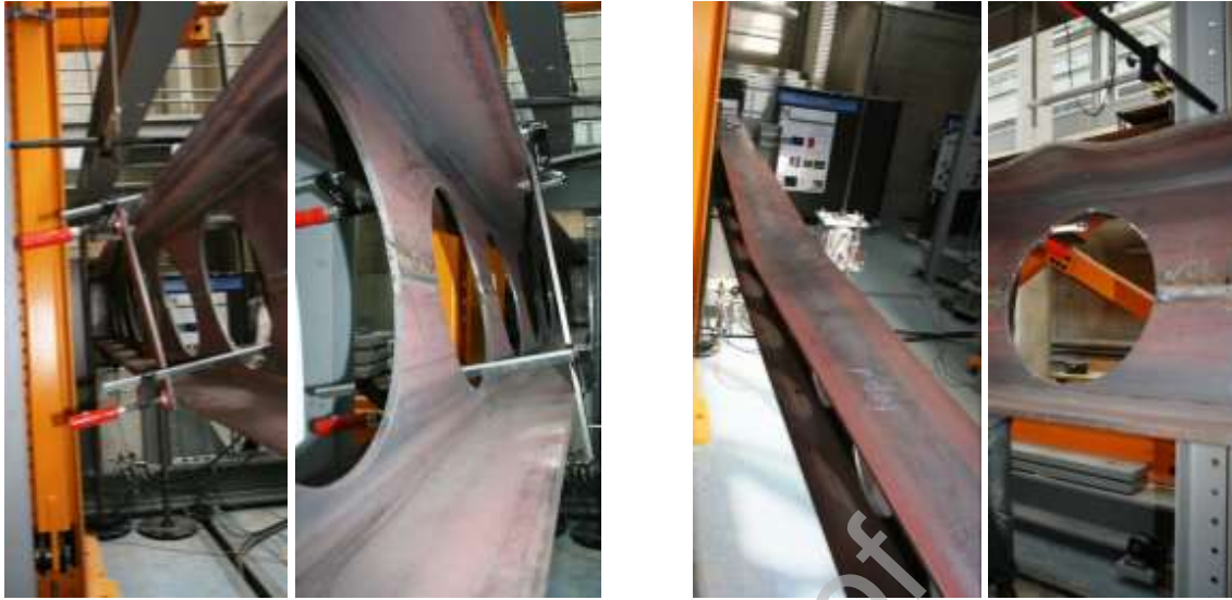
Fig. 12: Deformed configuration & torsional twist at peak load and residual deformation after unloading (HEA 340 specimen).
