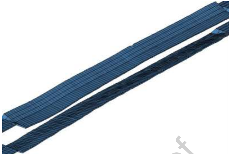
Fig. 8: Initial geometrical imperfection in web and flanges (magnified 20 times, base profile: HEA 340).
