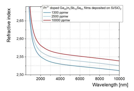
Figure 2: Refractive index spectral dependences of  $Pr^{3+}$  doped GeInSbSe thin films with different doping level (1300, 2500 and 10,000 ppmw).
