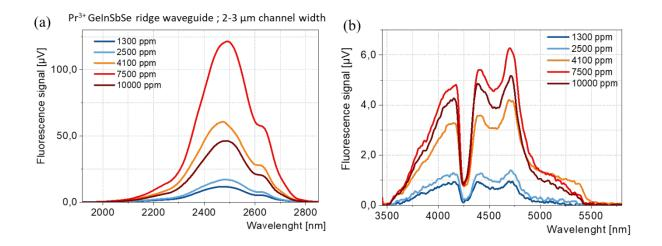
Figure 5. Averaged (a) SWIR and (b) MWIR emissions measured for  $Pr^{3+}$  doped GeInSbSe ridge waveguides widths of 2.0, 2.5 and 3.0  $\mu m$ .
