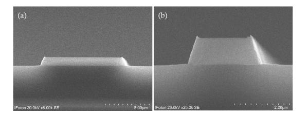
Figure 7. SEM images of 7500 ppmw. Pr³+: GeInSbSe waveguide of (a) 9  $\mu$ m and (b) 2  $\mu$ m width.
