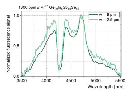
Figure 6. MWIR luminescence from 1300 ppmw. doped Pr³+ GeInSbSe single mode waveguides signal compared to multimode waveguides.
