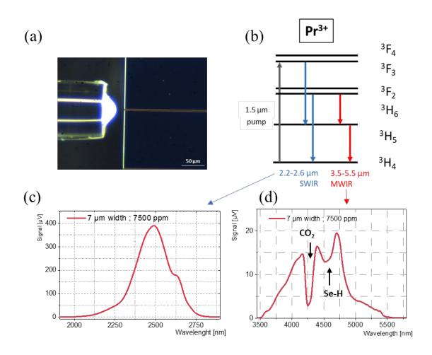
Figure 4. (a) optical microscope observation of the in-coupling region showing the lensed fiber and a 3- $\mu$ m wide channel waveguide; (b)  $Pr^{3+}$  simplified energy diagram for the SWIR and MWIR emissions; (c) SWIR and (d) MWIR luminescence of a 7  $\mu$ m wide 7500 ppmw.  $Pr^{3+}$  doped GeInSbSe ridge waveguide.
