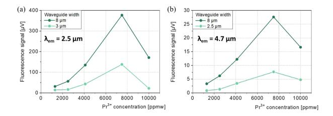
Figure 8. Maximum emission intensities recorded in the (a) SWIR (2.5  $\mu$ m) and (b) in the MWIR (4.7  $\mu$ m), for the 8  $\mu$ m and 2.5  $\mu$ m wide channels, as a function of the Pr³+ concentration in the GeInSbSe waveguide.
