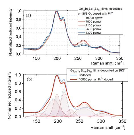
Figure 1: (a) Normalized reduced Raman spectra of the  $Pr^{3+}$ :  $Ge_{20}In_5Sb_{10}Se_{65}$  thin films for various  $Pr^{3+}$  concentrations deposited on Si substrates; (b)  $Pr^{3+}$  doped and undoped  $Ge_{20}In_5Sb_{10}Se_{65}$  films deposited from single undoped and 10,000 ppmw. doped cathodes on BK7 substrates.
