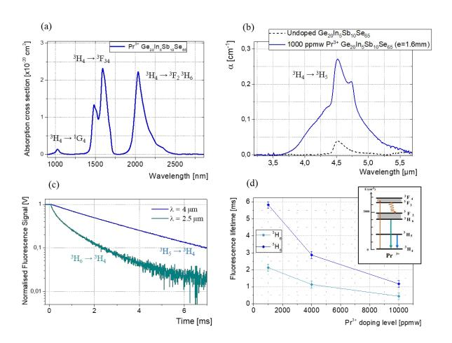
Figure 3. (a) Absorption cross section calculated from the 1000 ppmw.  $Pr^{3+}$  GeInSbSe in the SWIR and (b) absorption coefficient in the MWIR domains; (c) fluorescence decays recorded in the SWIR and MWIR for the 1000 ppmw. doped glasses; (d) Fluorescence lifetime for the  $Pr^{3+}$   $^3H_6$  and  $^3H_5$  manifolds as a function of  $Pr^{3+}$  concentration in bulk glasses and  $Pr^{3+}$  simplified energy diagram (inset).
