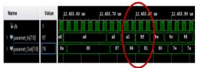
Fig.12. The test bench of the Image Luminance block.
