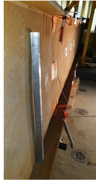
b) Post-peak web distortion of U-MS
