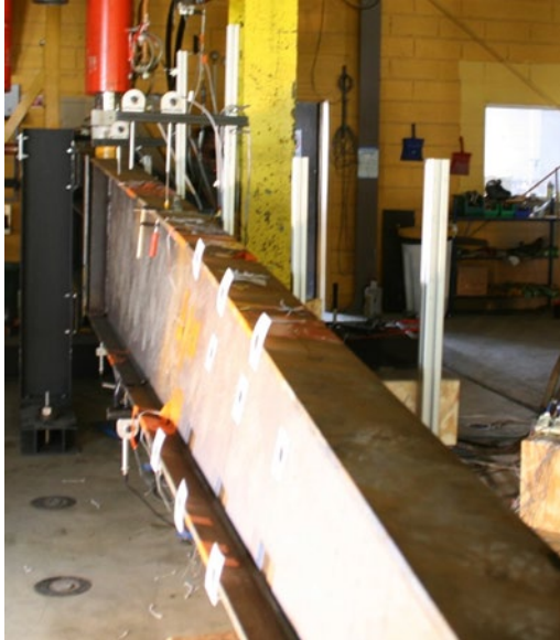
a) Lateral-torsional buckling of T-MS
