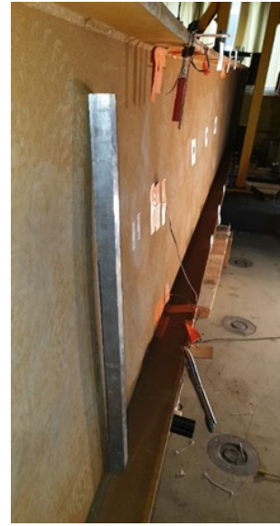
b) Post-peak web distortion of U-MS
