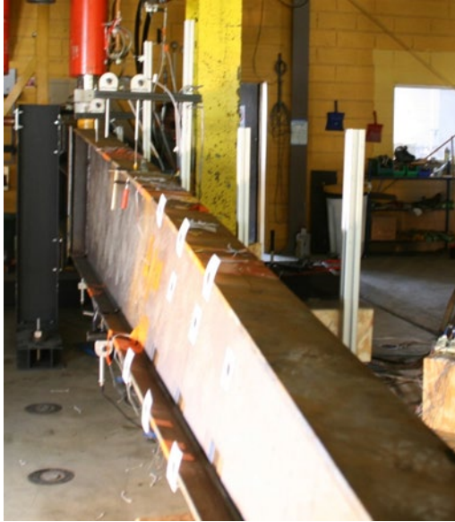
a) Lateral-torsional buckling of T-MS
