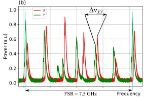
**Fig. 2.** Polarization-resolved optical spectrum observed with: (a) An optical spectrum analyzer, showing two combs associated with x (red) and y (green) eigenstates; (b) Fabry-Perot scanning interferometer (FPI) revealing the small detuning due to the residual birefringence of the laser. FSR: Free Spectral Range of the FPI.
