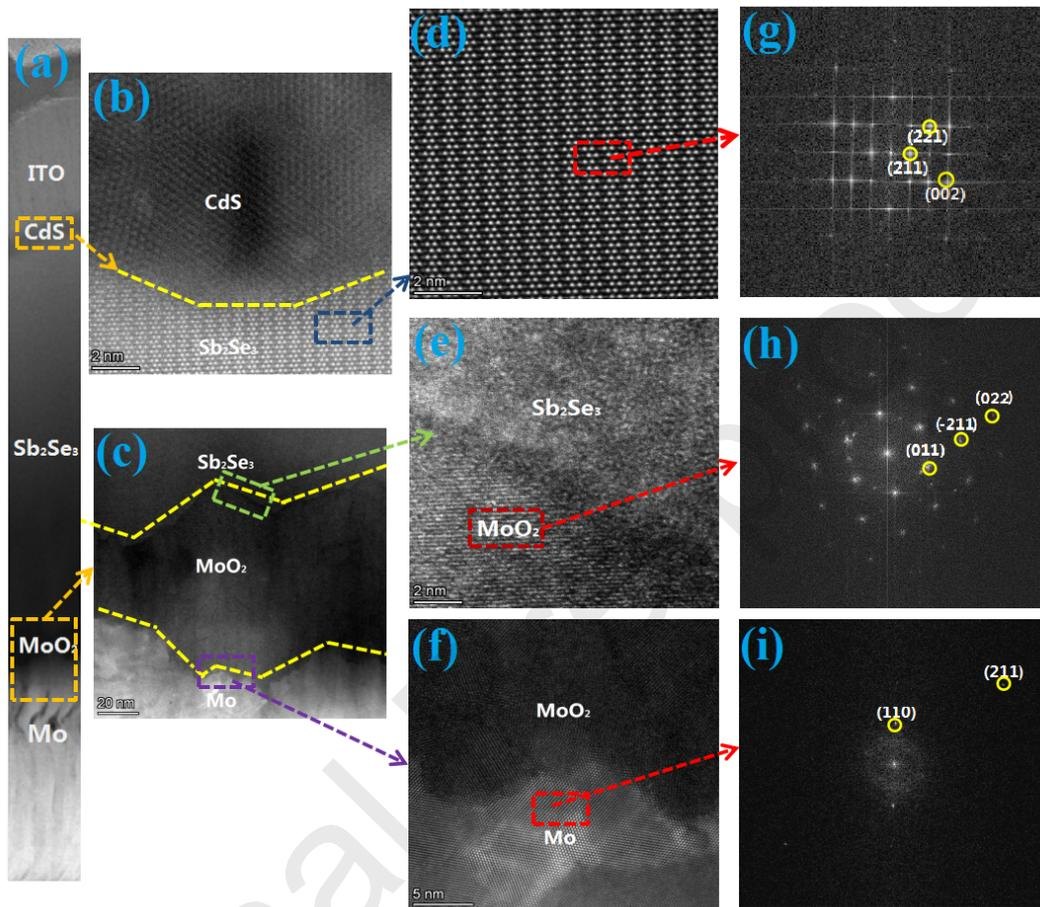
**Fig. 3.** (a) Cross-sectional TEM image of  $S_{Mo_2}$  device. (b)  $Sb_2Se_3$ /CdS interface TEM image. (c) Mo/ $MoO_2$ / $Sb_2Se_3$  back contact TEM images. (d-f) High-resolution TEM images of  $Sb_2Se_3$  absorber layer,  $MoO_2/Sb_2Se_3$  interface, and Mo/ $MoO_2$  interface. (g-i) The SAED patterns of  $Sb_2Se_3$  absorber layer,  $MoO_2/Sb_2Se_3$  interface, and Mo/ $MoO_2$  interface.
