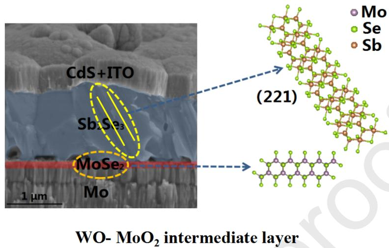
**Fig. S3.** Cross-sectional SEM image of S<sub>Mo1</sub> device (WO-MoO<sub>2</sub> intermediate layer)
