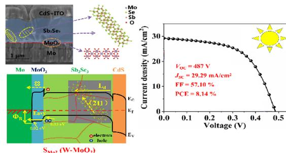
The  $MoO_2$  intermediate layer enhanced the growth of (211) oriented  $Sb_2Se_3$  absorber and the transport of photo-generated hole at the back contact. The power conversion efficient (PCE) of  $Sb_2Se_3$  solar cell was improved to 8.14 %.
