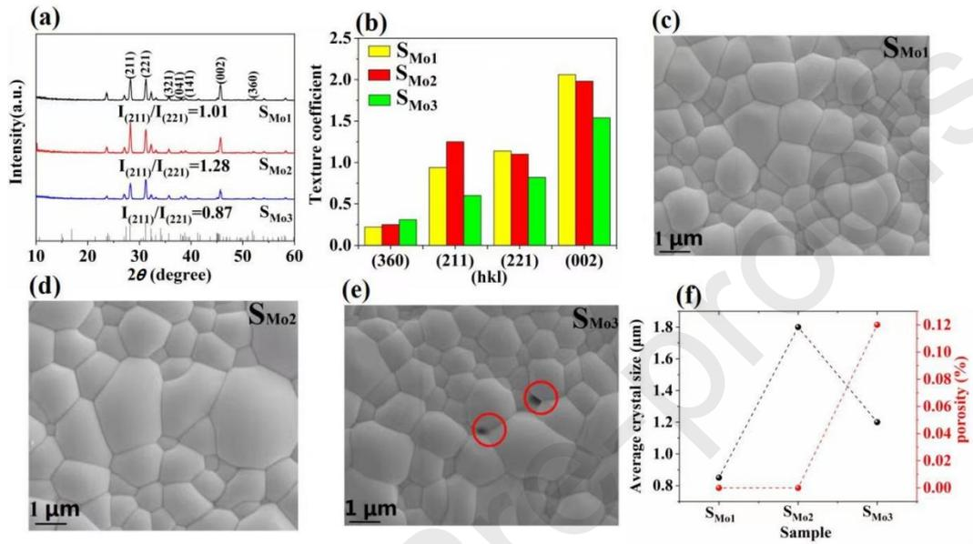
**Fig. 2.** (a) XRD patterns of  $\text{Sb}_2\text{Se}_3$  thin films. (b) Texture coefficients of the diffraction peaks of  $\text{Sb}_2\text{Se}_3$  thin films. (c-e) Surface morphologies of  $\text{Sb}_2\text{Se}_3$  thin films. (f) The average crystal sizes and porosity of  $\text{Sb}_2\text{Se}_3$  thin films.
