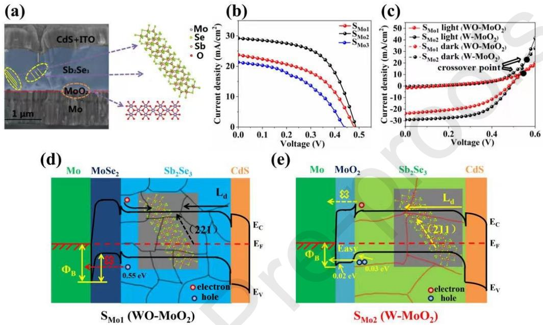
**Fig. 1.** (a) Cross-sectional SEM image of  $S_{Mo2}$  device. (b)  $J$ - $V$  curves of  $S_{Mo1}$ ,  $S_{Mo2}$  and  $S_{Mo3}$  devices. (c)  $J$ - $V$  curves of  $S_{Mo1}$  and  $S_{Mo2}$  devices under light and dark states. (d) The band diagrams of  $S_{Mo1}$ . (e) The band diagrams of  $S_{Mo2}$  devices.
