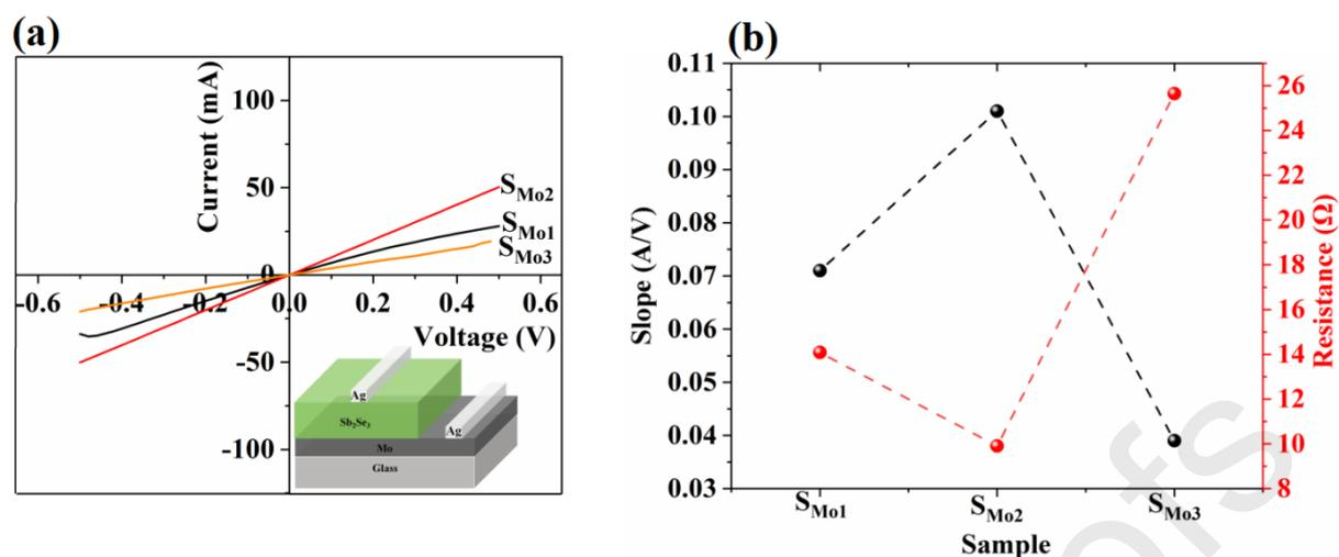
**Figure S8.** (a) *I-V* curves of Mo/ $Sb_2Se_3$  back contact (the schematic diagram of structure used to test *I-V* curves was inserted). (b) The slopes and resistance curves of  $S_{Mo1}$ ,  $S_{Mo2}$ , and  $S_{Mo3}$  samples.
