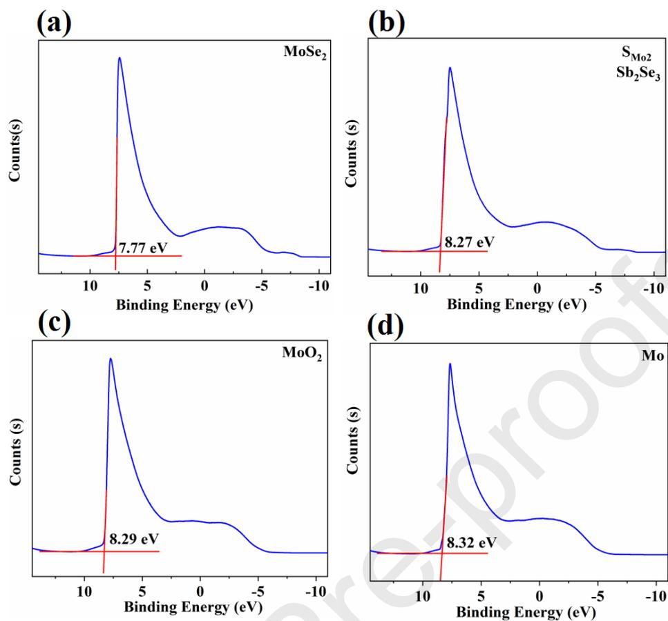
**Fig. S5.** UPS spectra for (a) the surface of  $\text{MoSe}_2$  interface layer, (b) the back of  $\text{Sb}_2\text{Se}_3$  layer in  $\text{S}_{\text{Mo}_2}$  device, (c) the surface of  $\text{MoO}_2$  intermediate layer, and (d) the surface of  $\text{Mo}$ .
