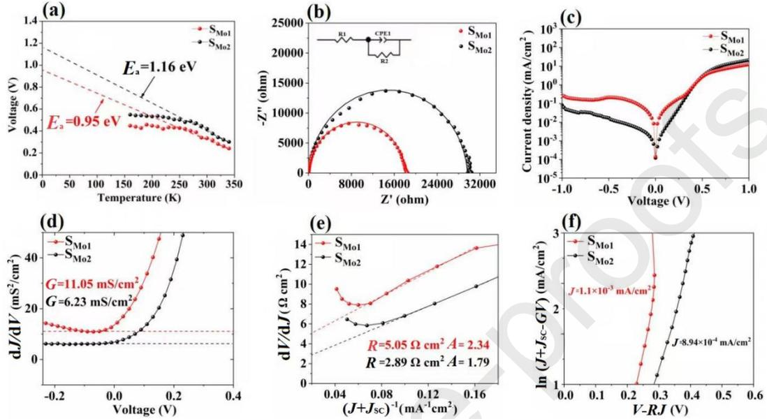
**Fig. 6.** (a) Temperature-dependent  $V_{OC}$  measurements. (b) Nyquist plots of  $S_{Mo1}$  and  $S_{Mo2}$  devices. (c) Dark  $J$ - $V$  curves of  $S_{Mo1}$  and  $S_{Mo2}$  devices. (d) Shunt conductance  $G$  of  $S_{Mo1}$  and  $S_{Mo2}$  devices. (e) Series resistance  $R$  and ideality factor  $A$  of  $S_{Mo1}$  and  $S_{Mo2}$  devices. (f) Reverse saturation current density  $J_0$  of  $S_{Mo1}$  and  $S_{Mo2}$  devices.
