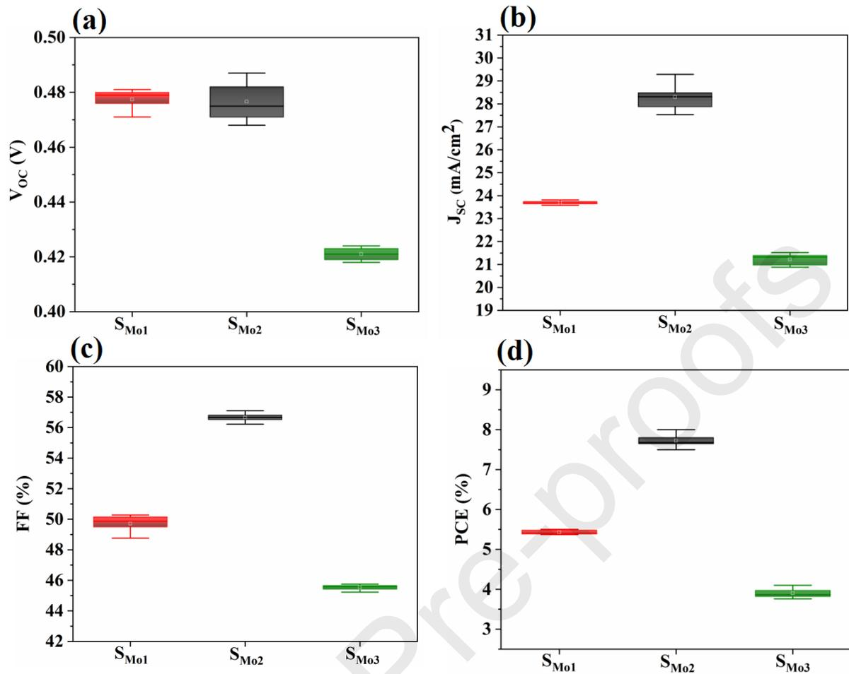
**Fig. S4.** Statistical distribution of the devices performance parameters including (a) open-circuit voltage ( $V_{OC}$ ), (b) short-circuit current density ( $J_{SC}$ ), (c) fill factor (FF), and (d) power conversion efficiency (PCE).
