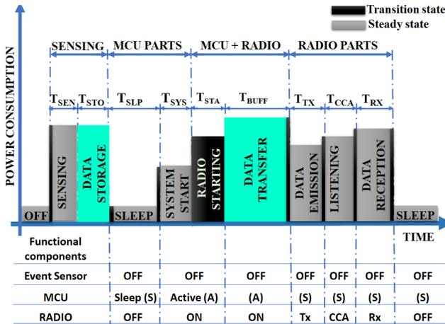
Fig. 2: WSD operation phases and timing periods scheme.
