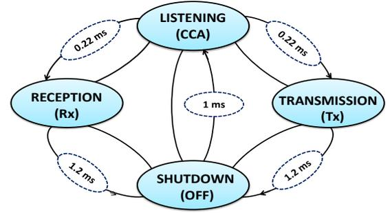
Fig. 3: CC2420 State and Transition Diagram [52]
