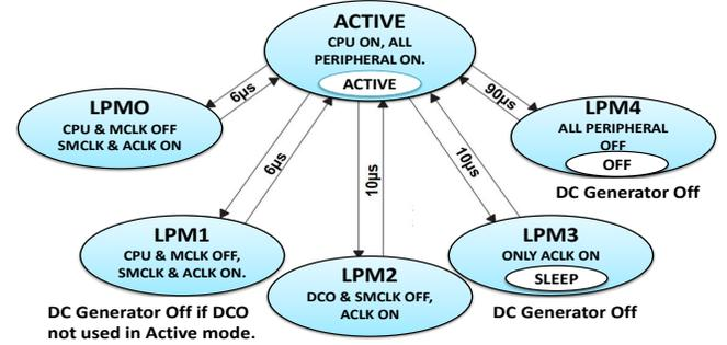
Fig. 4: MCU inter-mode and its transition time duration [54]
