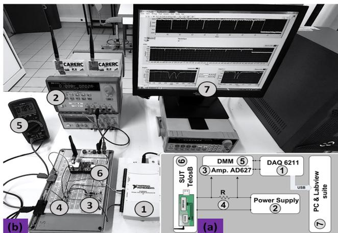
Fig. 5: Experimental setup (a) synoptic and (b) photo.
