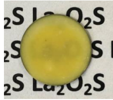
Fig. 11. Photograph of \text{La}_2\text{O}_2\text{S} translucent ceramic sintered at 1250^\circ\text{C} (Thickness = 0.5 mm)
