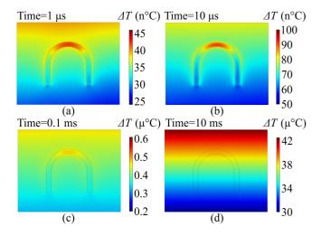
**FIGURE 5.**  $\Delta T$  distribution within capillary for *IPD* = 10 W/m<sup>2</sup> at 60 GHz: (a) 1  $\mu$ s; (b) 5  $\mu$ s; (c) 0.1 ms; (d) 10 ms.
