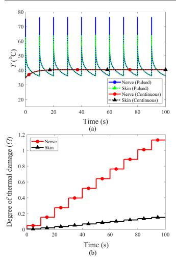
**FIGURE 8.** (a) Time course of temperature within nerve and surrounding skin due to continuous (*IPD* = 4.02 kW/m<sup>2</sup>) and pulsed (ten 3  $\mu$ s-pulses with *IPD* = 13.4 GW/m<sup>2</sup> separated by a cooling period of 10 s each) exposure at 60 GHz; (b) thermal damage within nerve and surrounding skin calculated for 10 s periods.
