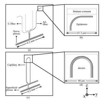
**FIGURE 1.** Geometric model: (a) cutaneous nerves; (b) terminal section of Aδ fiber; (c) cutaneous blood vessels; (d) capillary loop.
