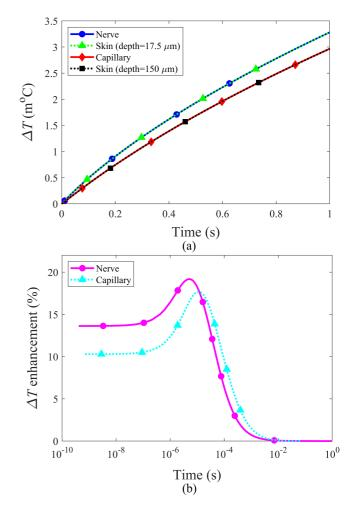
**FIGURE 3.** (a) Time course of  $\Delta T$  within nerve, capillary and surrounding skin; (b)  $\Delta T$  enhancement within nerve and capillary. (*IPD* = 10 W/m<sup>2</sup> at 60 GHz).
