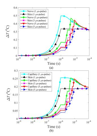
**FIGURE 7.**  $\Delta T$  for 1  $\mu$ s, 3  $\mu$ s and 5  $\mu$ s-mmWave pulses with constant fluence of 0.48 kJ/m<sup>2</sup> (*IPD* = 480 MW/m<sup>2</sup>, 160 MW/m<sup>2</sup> and 96 MW/m<sup>2</sup>): (a) nerve; (b) capillary.
