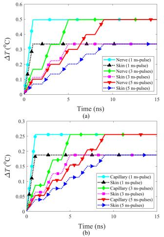
**FIGURE 6.**  $\Delta T$  for 1 ns, 3 ns and 5 ns mmWave pulses with constant fluence of 0.48 kJ/m<sup>2</sup> (*IPD* = 480 GW/m<sup>2</sup>, 160 GW/m<sup>2</sup> and 96 GW/m<sup>2</sup>): (a) nerve; (b) capillary.
