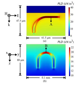
**FIGURE 2.** *PLD* distribution for *IPD* = 10 W/m<sup>2</sup> at 60 GHz: (a) A $\delta$  nerve fiber; (b) capillary loop.
