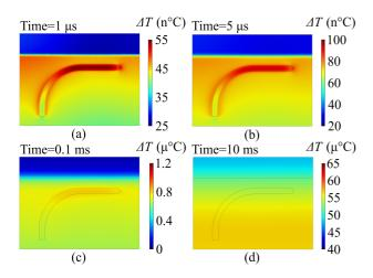
**FIGURE 4.**  $\Delta T$  distribution within nerve for *IPD* = 10 W/m<sup>2</sup> at 60 GHz: (a) 1  $\mu$ s; (b) 5  $\mu$ s; (c) 0.1 ms; (d) 10 ms.
