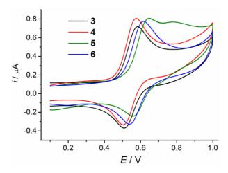
**Figure 3.** Cyclic voltammograms of complexes **3-6** recorded at a glassy carbon working electrode in DMF containing 0.1 M [n-Bu<sub>4</sub>N][PF<sub>6</sub>] at T = 298 K with a sweep rate v = 0.1 V s<sup>-1</sup>, reference electrode Ag/AgCl. The second redox event observed in the Zn<sup>II</sup> complex **5** could be attributed to an adsorption process.
