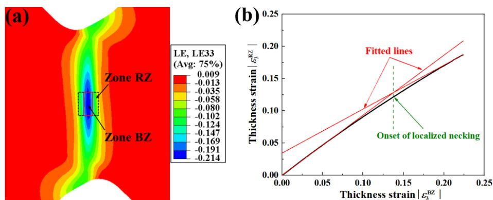
**Figure 5.** (a) Thickness strain field of specimen II under uniaxial tensile strain state, and selection of zones BZ and RZ. (b) Determination of onset of localised necking based on the CRIT4.
