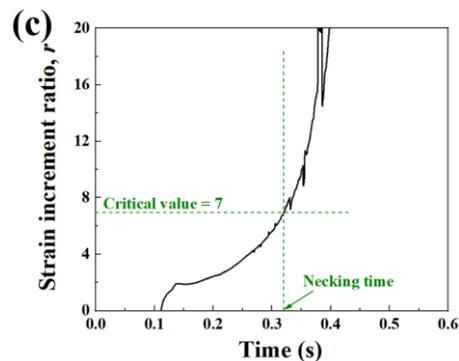
**Figure 4.** (a) Equivalent plastic strain field of specimen II under plane strain condition, (b) evolutions of the equivalent plastic strain in Elements A and B, (c) evolution of the equivalent strain increment ratio.
