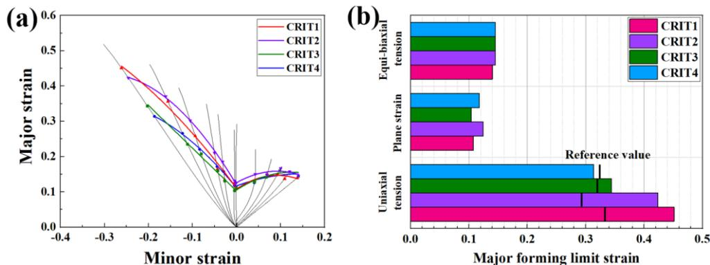
**Figure 6.** (a) The predicted FLCs of AA6061-T4 determined with different necking criteria, (b) the major forming limit strains for three representative strain states.
