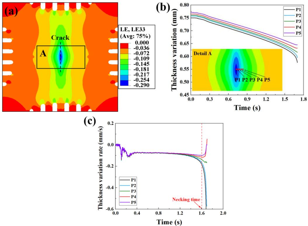
**Figure 3.** (a) The thickness strain field of specimen I under the biaxial tensile ratio of  $V_{L1}/V_{L2} = 1/0.4$  (mm/s), (b) thickness variations of the five points, (c) determination of necking time based on the CRIT2.
