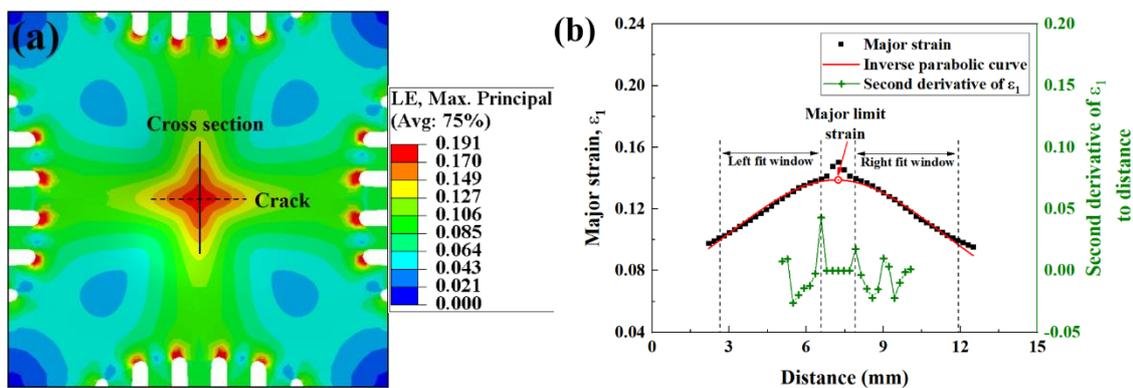
**Figure 2.** (a) The major strain field of specimen I under equi-biaxial loading condition, (b) determination of the major limit strain based on the CRIT1.
