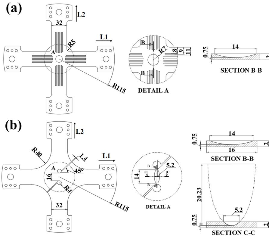
Figure 1. Dimensions of the used cruciform specimens (unit: mm): (a) Specimen I, (b) specimen II
