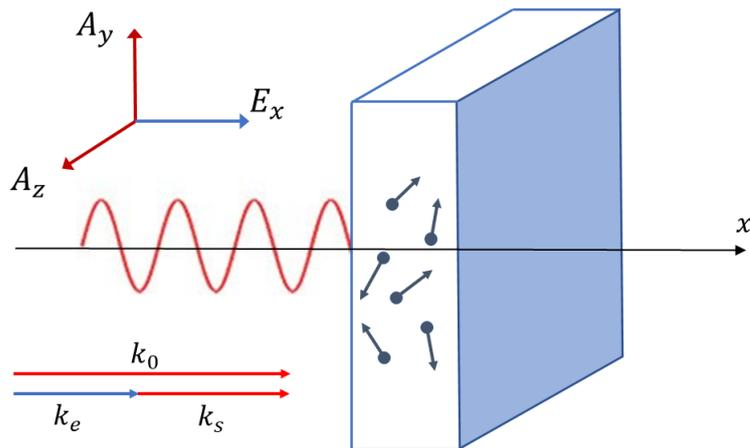
FIG. 1: Schematic view of our 1D configuration for SRS. All fields depend only on the longitudinal variable  $x$ . The electromagnetic wave is fully characterized by a transverse vector potential  $\mathbf{A}_\perp = (A_y, A_z)$  and a longitudinal electrostatic field  $E_x$ . The wave vectors and frequency of the incident, scattered, and electromagnetic waves must obey the matching relations (10).
