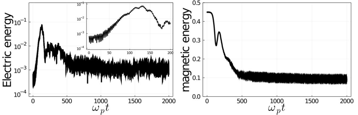
FIG. 2: Electrostatic energy  $\frac{\epsilon_0}{2} \int E_x^2 dx$  (left frame) and magnetic energy  $\frac{1}{2\mu_0} \int |\mathbf{B}_\perp|^2 dx$  (right frame) as a function of time. The inset shows a zoom of the electrostatic energies at short times, evidencing the exponential growth of the Raman instability. Both energies are expressed in units of  $mc^2$ .
