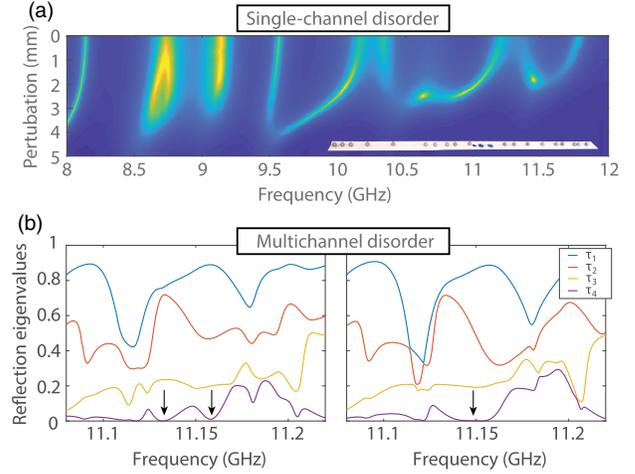
FIG. 3. (a) Color scale representation of  $R(\nu, z)$  for a symmetric single-channel disordered medium. The inset shows a picture of metallic spheres inserted within the waveguide. (b) Spectra of reflection eigenvalues  $[\tau_1(\nu), \dots, \tau_4(\nu)]$  in a multichannel disordered cavity in the underperturbed regime (left) and tuned at an RL EP (right). The arrows indicate the frequency of the coalescing zeros of  $\tau_4(\nu)$ .
