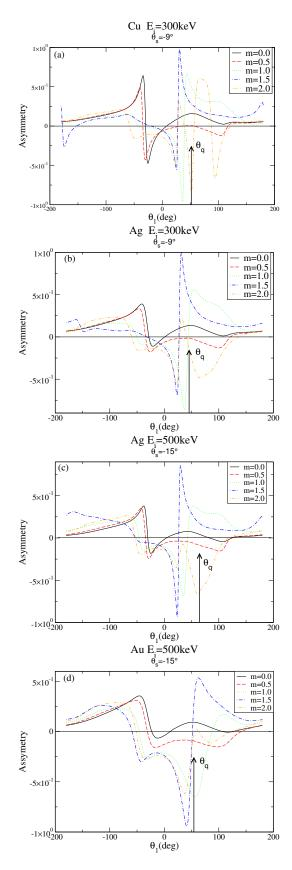
FIG. 6: Spin asymmetry A in TDCS for Cu(a),  $Ag(E_i = 300 \text{keV} \text{ and } E_i = 500 \text{keV})((b) \text{ and } (c))$  and Au(d) respectively. Other kinematical variables are same as Fig.4 and Fig.5
