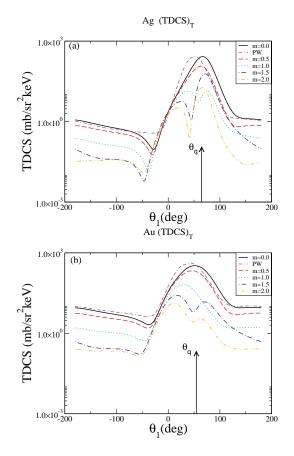
FIG. 5:  $(TDCS)_T$  for Ag  $(E_i = 500 \text{keV}, E_s = 375 \text{keV}, E_1 = 100 \text{keV})$  and Au  $(E_i = 500 \text{keV}, E_s = 310 \text{keV}, E_1 = 100 \text{keV})$  targets for given m's with  $\theta_s = -15^{\circ}$  and  $\theta_p = 15^{\circ}$ . Here  $(TDCS)_0$  for plane wave calculation  $(\theta_p = 0, m = 0)$  is represented by dashed-dotted-dashed line.
