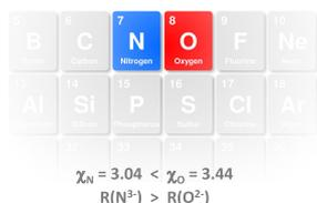
Effect nitrogen insertion on the optical gap (d<sup>0</sup> metal)
