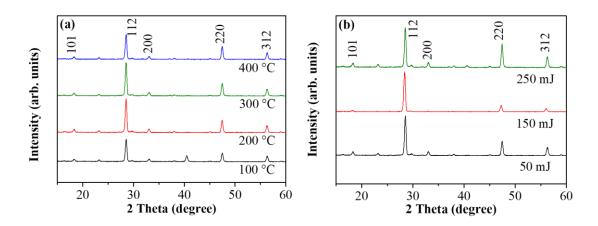
**Figure S5.** XRD of the CZTS thin films fabricated by (a)different substrate temperature and (b)different laser energy pulse.
