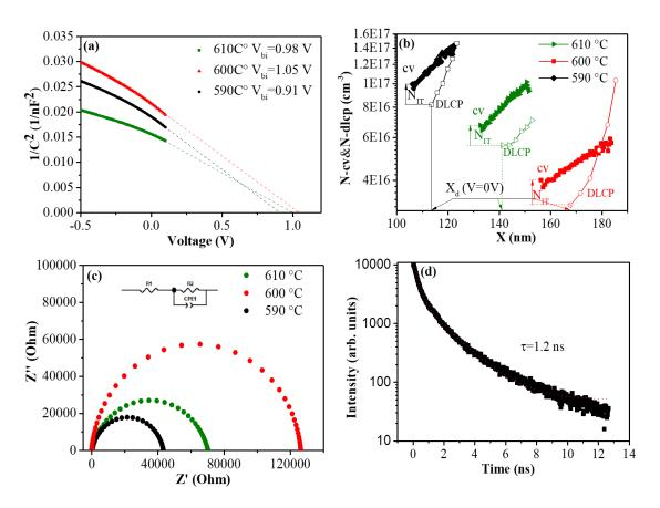
**Figure 5**. (a)  $1/C^2 - V$  plots, (b) CV and DLCP profiles, (c) EIS Nyquist plots of the devices with different annealing temperatures under a 0v bias, (d) TR - PL curves of CZTS solar cells.
