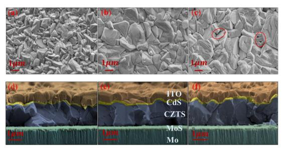
**Figure 3**. SEM top-view images of the CZTS thin-films with different post-sulfurization heat treatment temperatures, (a) 590 °C, (b) 600 °C, (c) 610 °C, respectively. SEM cross section images of the CZTS thin-films with different post-sulfurization heat treatment temperatures, (d) 590 °C, (e) 600 °C, and (f) 610 °C. The length of red scale bar at the left bottom of each image represents 1μm.
