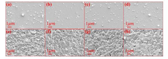
**Figure S4.** SEM of the precursors prepared with different substrate temperatures (a.100  $^{\circ}$ C, b. 200  $^{\circ}$ C, c. 300  $^{\circ}$ C, d. 400  $^{\circ}$ C) and the corresponding CZTS film morphology beneath, sulfurized at 600  $^{\circ}$ C.
