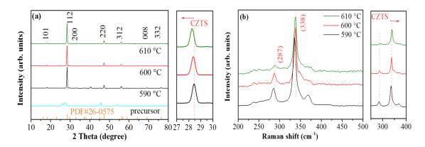
**Figure 2**. (a) The X-ray diffraction (XRD) patterns and (b) Raman spectra of the CZTS thin films with different post-sulfurization temperatures. The enlargement of the (112) diffraction peak of the films is shown in (a) right, enlargement of the Raman shift at 287 cm<sup>-1</sup> and 337 cm<sup>-1</sup> is shown in (b) right.
