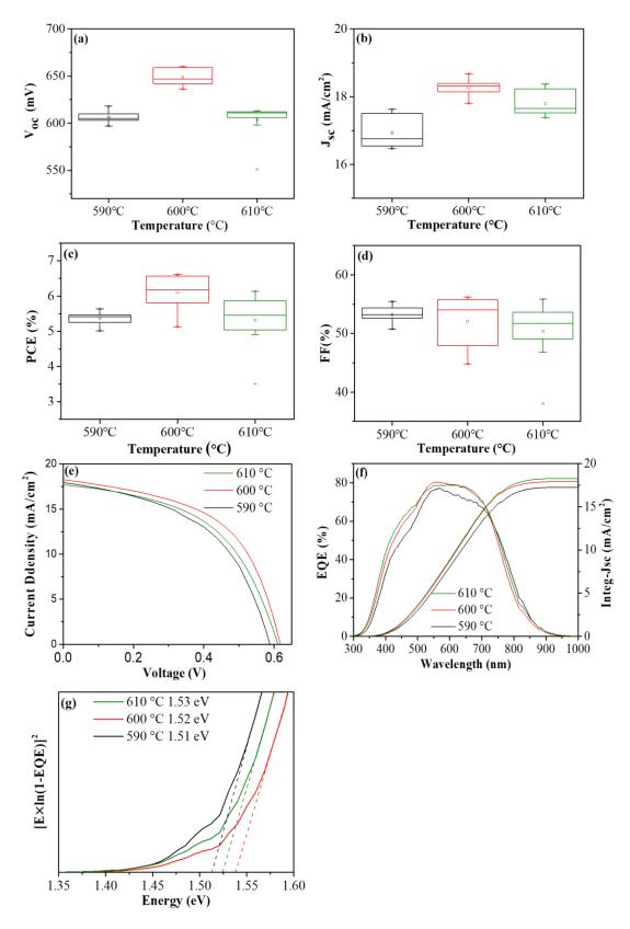
**Figure 4**. (a)-(d) Statistical box plot of devices performance parameters for 16 solar cells obtained from each variety of absorber film fabricated at different temperatures, (a) open-circuit voltage  $(V_{OC})$ , (b) short-circuit current density  $(J_{SC})$ , (c) power
