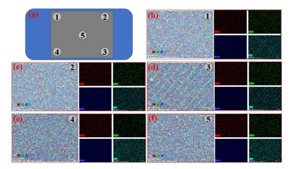
**Figure S6.** Chemical composition mapping of five point for as-deposition film fabricated by PLD. (a) Schematic diagram of the test location points on precursor. (b)-(f) Composition mapping of the corresponding points.
