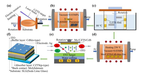
**Figure 1**. Schematic illustration of the preparation process of the Cu<sub>2</sub>ZnSnS<sub>4</sub> thin film solar cell. (a) CZTS precursor thin film deposition by PLD, (b) post-sulfurization heat treatment to obtain CZTS thin film, (c) deposited CdS buffer layer via CBD, (d) post-annealing of the CZTS/CdS heterojunction, (e) deposited ITO layer by magnetron sputtering, (f) final structural representation of the CZTS thin film solar cell.
