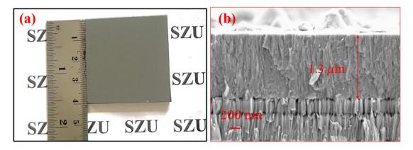
**Figure S1.** The  $4 \times 4$  cm<sup>2</sup> precursor film photo (a) and SEM cross section images of the as-deposited CZTS thin-films (b)
