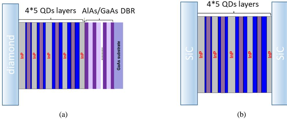
Fig. 3 : Schematic structures of the QD based VECSEL(a) and MECSEL(b)
