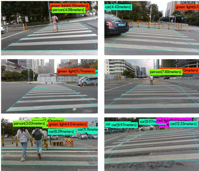
Fig. 13. Some examples of image output detected by the proposed system.
