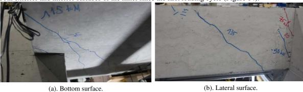
Figure 12. Test C1B: cracks due to punching shear.
