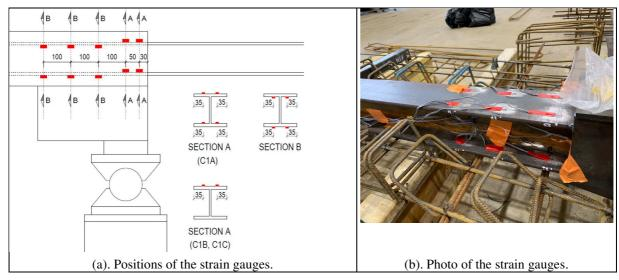
Figure 6. Strain gauges (dimensions in mm).
