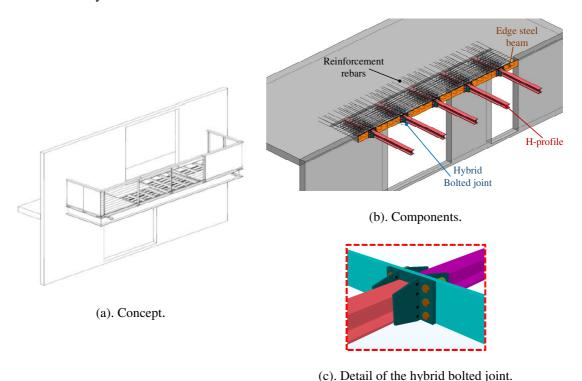
Figure 1. System of the innovative demountable steel balcony.
