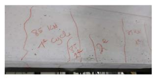
Figure 14. Test C1C: vertical cracks on the concrete lintel.
