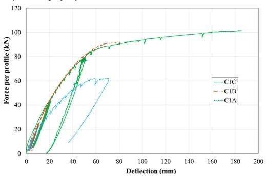
Figure 16. Deflection of the HEB120 profile at the applied load in function of force per profile.
