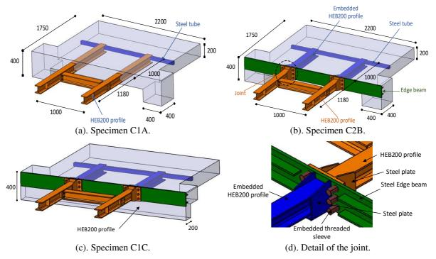
Figure 4. Test specimens (dimensions in mm).
