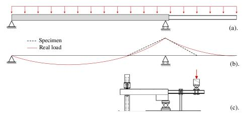
Figure 2. Specimen design: (a). Configuration of real loads on floor-to-balcony connection. (b). bending moment diagrams. (C). Configuration of testing.
