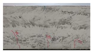
Figure 11. Test C1A: Vertical cracks at the middle span of the slab.
