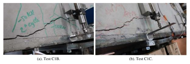
Figure 13. Crack due to the separation between the concrete slab and the steel edge beam.
