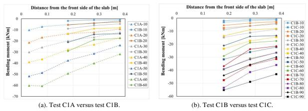
Figure 18. Distribution of bending moment in the embedded H-profile.
