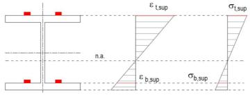
Figure 17. Strain and stress distribution over the height of the profile section within the elastic domain.
