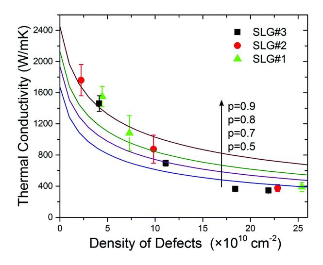
**Figure 3** Dependence of the TC on the density of defects of SLG. The experimental data are shown by squares, circles and triangles. The solid curves are calculated curves. p is a parameter called the specularity parameter; for p = 0 the scattering is fully diffuse and for p = 1, there is no extra thermal resistance due to diffusion. Reproduced with permission from ref. [36]
