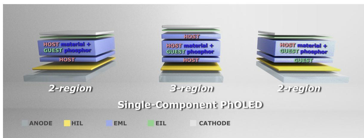
**Figure 15.** Schematic representation of Single-Component PhOLEDs with 3-region or 2-region
