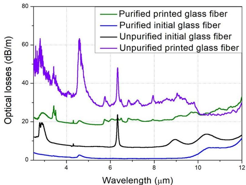
**Figure 6.** Attenuation spectra of the initial glasses (unpurified and purified glasses, red curve and blue curve respectively) and the “printed” glass fibers (from an unpurified glass and from a purified glass, purple and green respectively)
