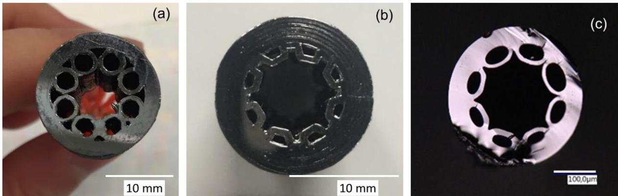
**Figure 8.** Printed preforms: (a) cross-section view of the chalcogenide printed 8 capillaries preform and (b) cross-section view of the chalcogenide printed 8 half-capillaries preform (c) cross section of a hollow core fiber drawn from the preform shown in (b).
