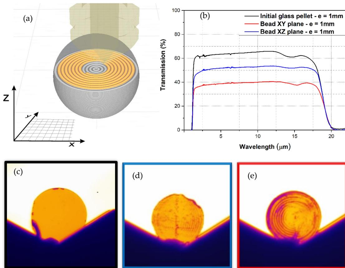
**Figure 5.** Optical transmission of printed beads: (a) numerical view of the 3D printing process, (b) initial glass transmission compared to the transmission of 2 disks cut in the XY plan (red curve) and XZ plan (blue curve), respectively. IR camera views in the 7–13  $\mu\text{m}$  window (c) initial TAS glass, (d) XZ plan, (e) XY plan.
