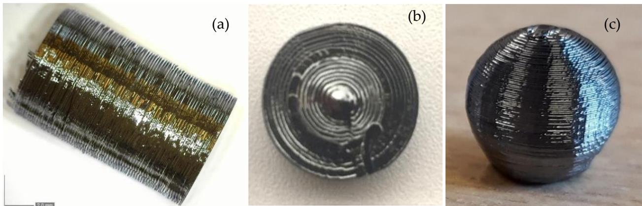
**Figure 3.** Chalcogenide 3D printed samples: (a) chalcogenide cylinder, (b) chalcogenide disk (c) chalcogenide bead.
