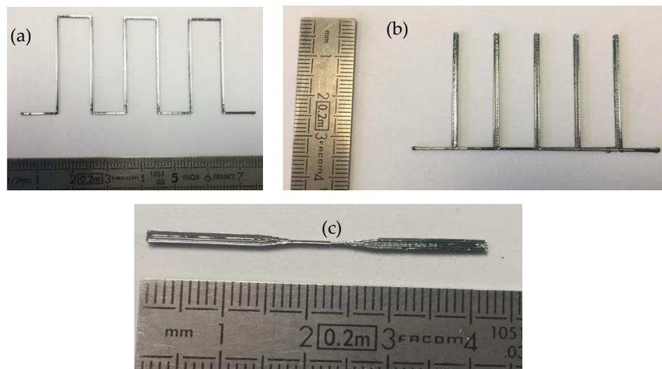
**Figure 7.** Linear 3D printed chalcogenide glass: (a) 700  $\times$  500  $\mu\text{m}$  slots shapes, (b) 1000  $\times$  800  $\mu\text{m}$  comb and (c) 1000  $\times$  250  $\mu\text{m}$  rectangular taper.
