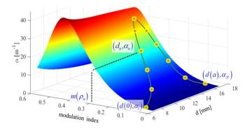
Fig.6. The colored surface represents the solution for  $\alpha$  of the local canonical problem for several modulation indexes *m* and periodicity values *d* at the amplitude control frequency  $\omega_p$ . For every periodicity and its corresponding radial distances  $\rho_n$  one selects the modulation index that provides the desired  $\alpha(\rho_n, \omega_p)$  value. All these  $\alpha(\rho_n, \omega_p)$  are represented by the yellow dots.
