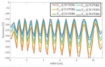
Fig.7. The color lines represent the  $X_{\rho\rho}$  component of the reactance tensor  $\underline{\mathbf{X}}(\rho,\omega)$  for different in-band frequencies  $\omega$  and along the  $\varphi = 0$  direction. The  $X_{\rho\rho}$  component is evaluated on a few frequency samples within the design bandwidth of the aperture.
