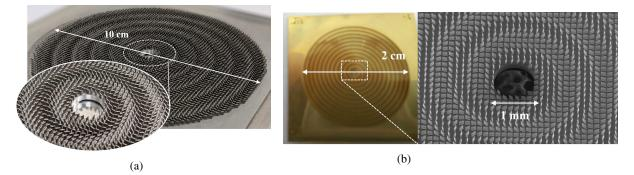
Fig. 2: (a) Ka-band modulated MTS antenna fabricated by metal additive manufacturing. (b) Modulated MTS antenna operating at 300 GHz and fabricated by DRIE.
