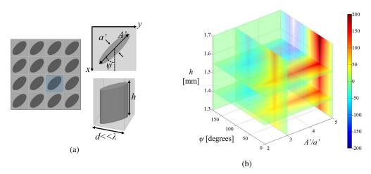
Fig. 1: (a) Description of the unit-cell geometry and local periodicity assumption. (b) Example of database relating the geometry of the unit-cell with the corresponding reactance tensor.
