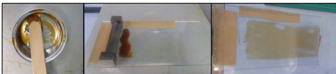
Figure S29. Illustration of the preparation of films derived from cured \alpha,\omega -[(EtO) 3 Si] 2 -PCOE/PPG* synthesized from the two-step ROIMP/CM Method II. From left to right: mixing of the SMP and the catalytic system (S1 (1wt%) and GF9 (1wt%)); formation of the film; the film after curing (Refer to the Experiential Section).
