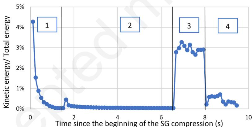
Figure 7: Temporal evolution of the ratio of the kinetic energy to total energy during the simulation steps: (1) SG compression, (2) SG deployment, (3) Removal of the delivery system from the left iliac artery and the stiff guidewires, and (4) Removal of the catheters.
