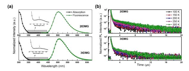
**Figure 2.** (a) UV-vis absorption, fluorescence (298 K) of **2tDMG** and **3tDMG** respectively. (b) Temperature-dependent PL decay curves from 300 to 100 K of **2tDMG** (40 wt%) and **3tDMG** (40 wt%) doped in DPEPO film respectively.
