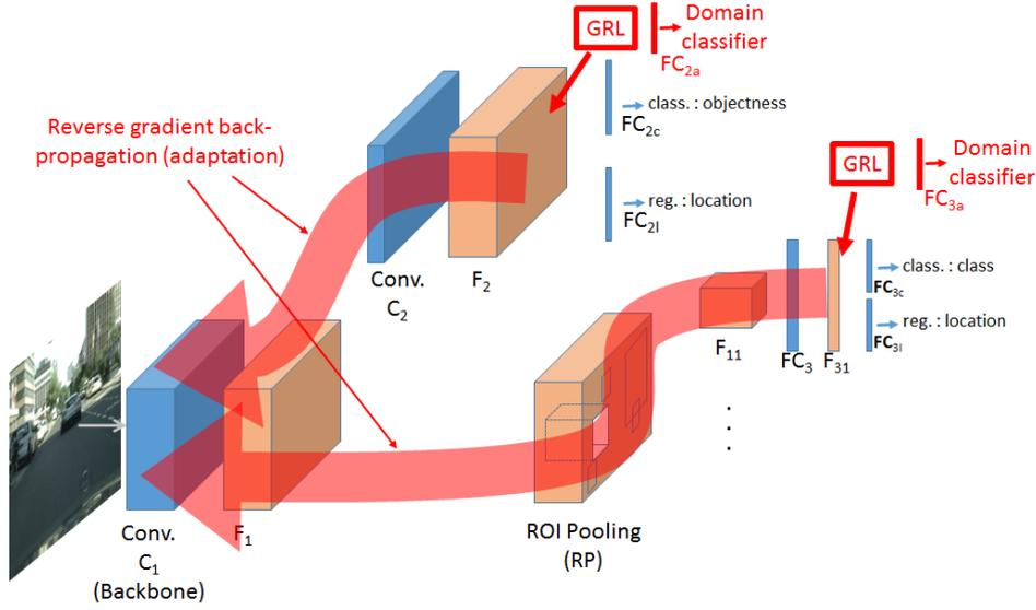
FIGURE 3 – Our domain adaptation for Faster R-CNN. See text for details
