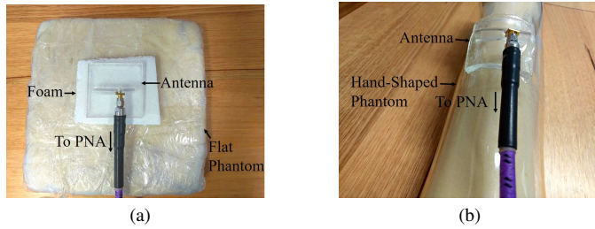
Fig. 12. Photographs of the antenna measurement set-ups: (a) on a flat phantom, (b) wrapped on a human-hand-shaped phantom.
