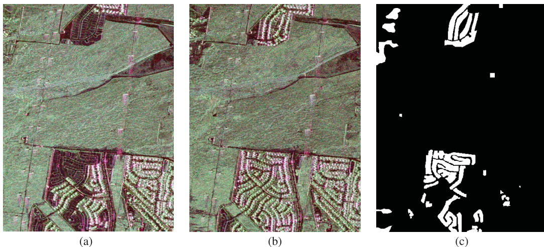
Fig. 8. UAVSAR images (in Pauli decomposition) on April 23, 2009 and May 11, 2015. (a) Before change, (b) after change, (c) ground truth, where white color is change and black color is no-change.
