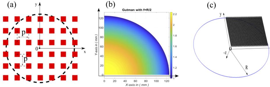
**Fig. 9.** (a)  $K \times K$  matrix designed for bottom metal pins with equal heights  $h$ , top view (b) index distribution along its quarter symmetric surface (c) 3D  $K \times K$  matrix with equal height bottom metal plates.
