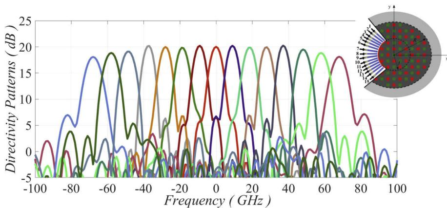
**Fig. 19.** Directivity patterns at center frequency  $f = 12.5$  GHz.
