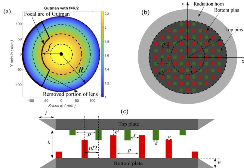
**Fig. 1.** (a) Effective refractive index  $n_{eff}$  of the Gutman Lens with focal arc  $f = R/2$ , (b) PPW GRIN Gutman lens layout using an IGS unit cell (top view), (c) 2D cut view,  $p=2.4$ ,  $a=0.8$ ,  $s=0.4$ ,  $h'=1.9$ ,  $h=4$ ,  $w=12$ , all dimensions in mm.
