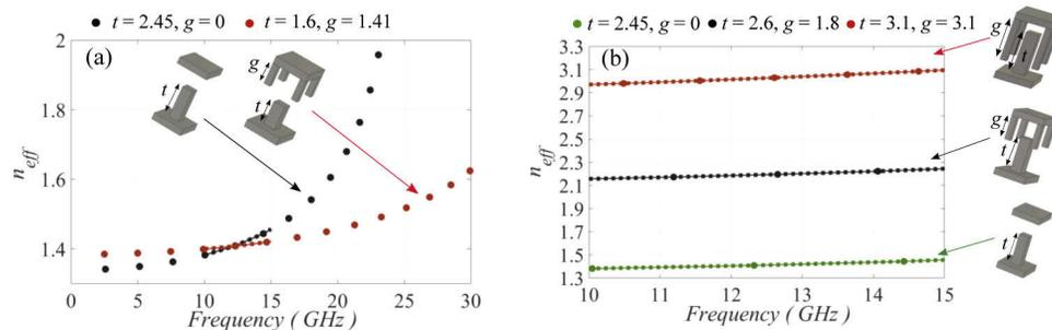
**Fig. 5.** Index comparison of (a) single pin unit-cell vs glide symmetry cell without interleaving (b) single pin unit cell vs glide symmetry cell with slight interleaving vs glide symmetry cell with maximum interleaving.
