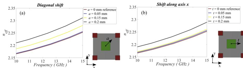
**Fig. 4.** Parametric study on the misalignments of the interleaved unit-cell (a) top pin diagonal shifting (b) top pin shifting along axis  $x$ .
