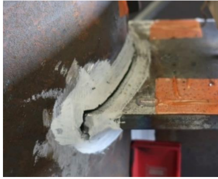
426 427 Fig. 11. LASTEICON_LC2 Failure: (a) beam-to-column connection tearing observed from 428 experiments, (b) von Mises equivalent plastic strains in the numerical model
