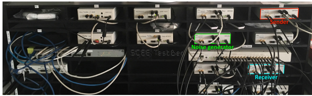
FIGURE 8. Example set-up used for our experiments, involving 3 separate USRPs synchronised through an octoclock.
