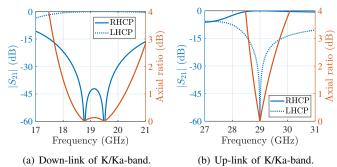
Fig. 4. Numerical results for the dual-band, orthogonally-polarized LP-to-CP converter with  $\phi_{01}^{xx} = 82.5^{\circ}$ . Axial ratio and transmission coefficients for both RHCP and LHCP are plotted in two bands: (a) 17-21 GHz and (b) 27-31 GHz.
