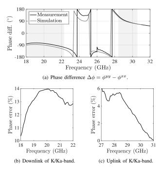
Fig. 11. (a) Phase difference  $\Delta \phi = \phi^{yy} - \phi^{xx}$  comparison between measurements and simulations. Percentage error of measured data in the (a) downlink and (b) uplink of the K/Ka-band.
