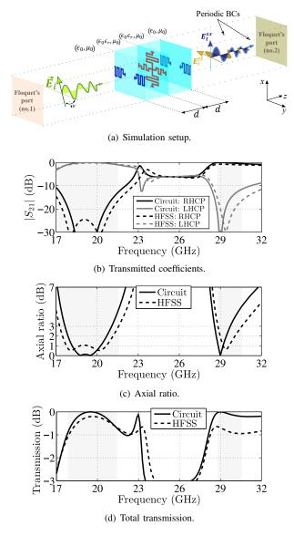
Fig. 7. (a) Simulation setup of the polarizer's unit cell. A comparison between the circuit network and full-wave simulations [36] is reported. (b) Transmitted LHCP and RHCP. (c) Axial ratio. (d) Total transmission. The full-wave simulations considers a normal incidence onto the polarizer. Besides, the incident E-field is linearly-polarized in the direction  $\hat{\alpha} = (\hat{x} \pm \hat{y})/\sqrt{2}$ .
