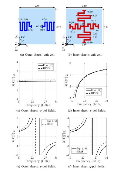
Fig. 6. Patterned metallic geometries of the metasurfaces' unit cell: (a) outer and (b) inner sheets. All dimensions are given in millimeters. The simulated susceptances for the patterned metallic geometries are shown in (c)-(e) for xand (d)-(f) for y-polarized fields. The black and grey dot markers indicate the desired design values at the frequency  $f_{01}$  and  $f_{02}$ , respectively.
