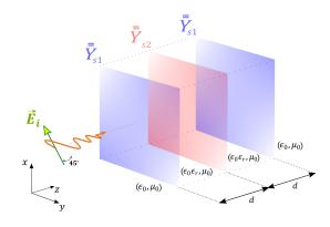
Fig. 2. Geometry of the problem under analysis. Three anisotropic sheet admittances are cascaded along the z-axis. The external sheet admittances are equal.
