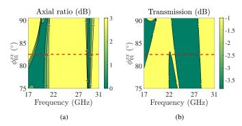
Fig. 3. Contour plots of the absolute value of (a) axial ratio and (b) transmission coefficient as a function of frequency and  $\phi_{01}^{xx}$ . The dashed red line indicates the chosen operating point for the design.
