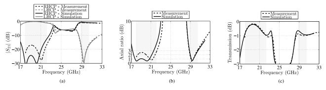
Fig. 10. Comparison between measured and full-wave performance of the polarizer. (a) Transmitted LHCP and RHCP. (b) Axial ratio. (c) Total transmission of the polarization converter. The measurements refer to a normal illumination of the DUT.
