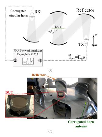
Fig. 9. (a) Schematic drawing of the experimental setup used to measure the polarizer: quasi-optical test-bench [39]. (b) Photograph of the test setup.
