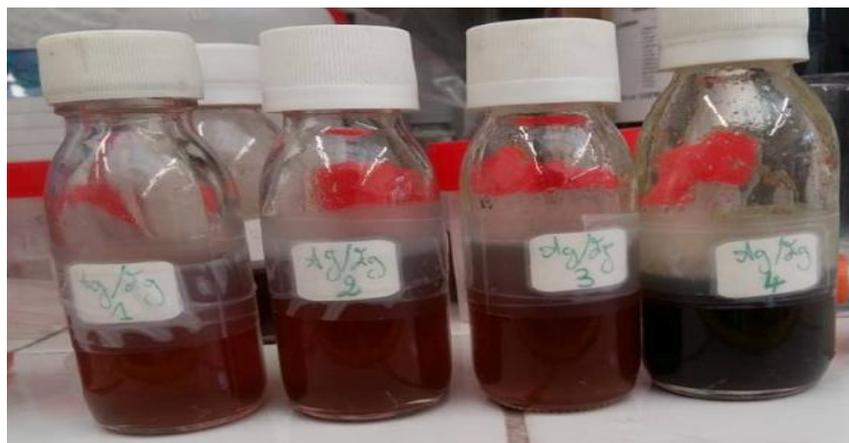
Figure 1: Photographs of the EGS-based nanofluids after Ag/EG synthesis prepared with different content of copolymer latex: (1) 99 mg, (2) 126 mg, (3) 305 mg, (4) 340 mg of copolymer latex, respectively.
