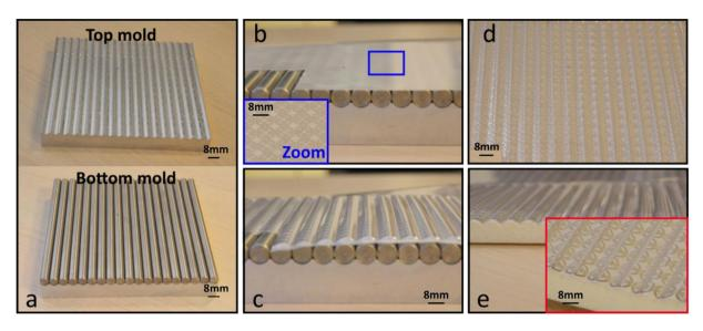
**Figure 3.** Optical image showing the main thermoforming process. (**a**) Top and bottom part of an aluminium mould; (**b**) the 2-D planar substrate placed on the bottom of the mould; (**c**) the substrates after the thermoforming step; (**d**) the wavy FSS patterns and (**e**) the thermoformed substrate placed on top of the 3-D object. The blue and red insets show higher resolutions of the patterns for screen printing and drop-on-demand printing, respectively.
