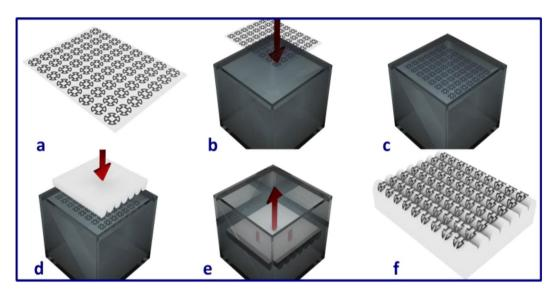
**Figure 4.** Fabrication of the FSS using WTP technology: (**a**) FSS patterns fabricated onto the 2-D planar PVA substrate; (**b**) depositing the substrate gently onto the water's surface; (**c**) the substrate floating on the water, allowing the hydrosoluble substrate to dissolve; (**d**) dipping the object through the floating patterns; (**e**) shaking and withdrawing the object; and (**f**) the final object conformally wrapped with the electronics.
