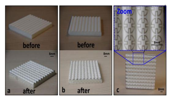
**Figure 5.** Optical images of the 3-D structure before and after the WTP process for the fabrication of the FSS prototype: (a) 45° oriented view, (b) 90° oriented view, (c) side view showing the top of the wave-shaped structure. The blue inset shows a higher resolution of the sub-patterns of the fabricated 3-D FSS.
