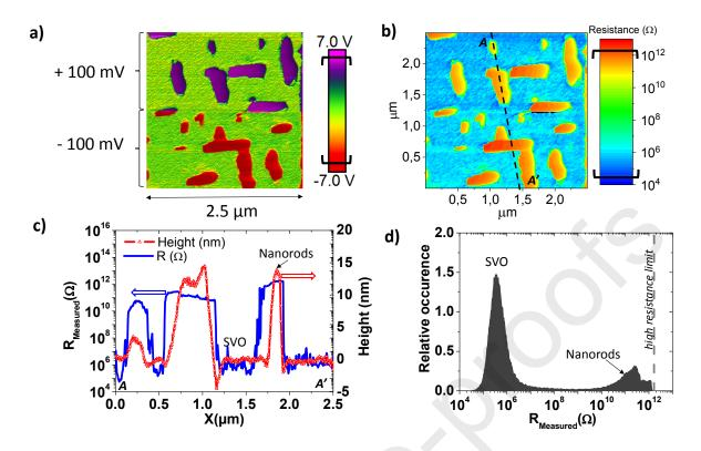
Figure 5. a) 2D-map of the V<sub>out</sub> signal from SSRM mode. b) 2D-map of the local resistance.c) Resistance profile along the line AA'. d) Resistance distribution in the scanned area. The brackets in the data scale indicate data threshold.
