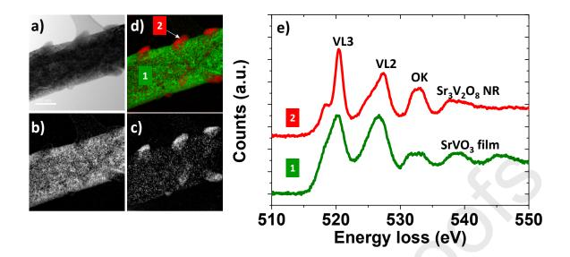
Figure 4. a) Bright field zero-loss TEM image showing a plane-view of a fraction of the SVO film with several elongated crystals. b) V<sup>4+</sup> state MLLS fit map of the same area.
