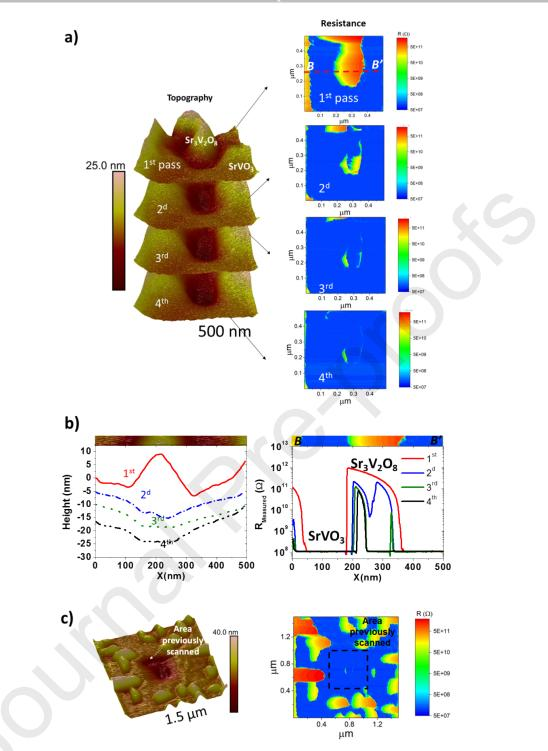
**Figure 6.** 3D-SSRM results (500 nm  $\times$  500 nm) for successive scans: a) AFM topography acquisitions and resistance maps for each scan. b) Line profiles of the topography and resistance along the line BB'. c) Topography and SSRM 2D-map of a larger scan 1.5  $\mu$ m x 1.5  $\mu$ m centered on the area previously scanned.
