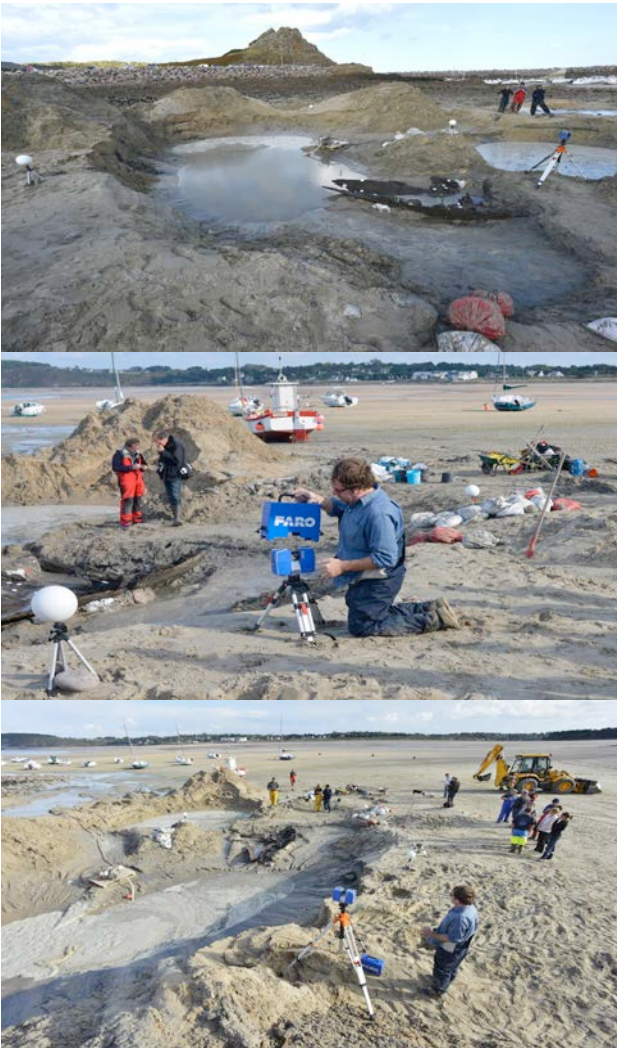
Figure 10. Wreck digitization with laser scanner (F.Osada/Drassm)
