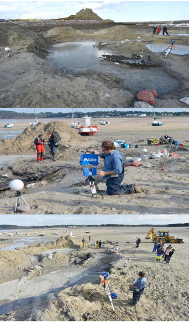
Figure 10. Wreck digitization with laser scanner (F.Osada/Drassm)
