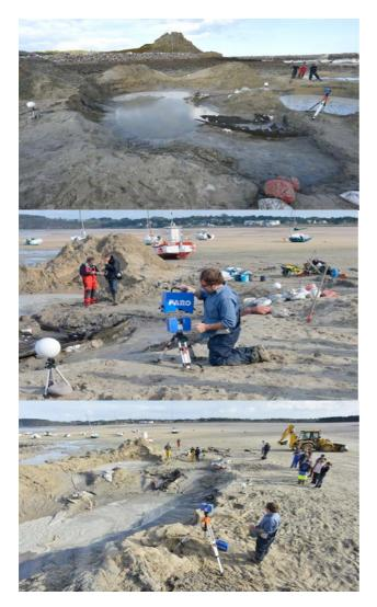
Figure 10. Wreck digitization with laser scanner (F.Osada/Drassm)
