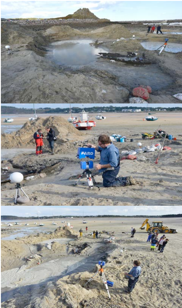
Figure 10. Wreck digitization with laser scanner (F.Osada/Drassm)
