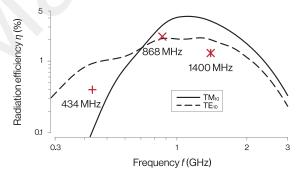
Fig. 5. Comparison of the proposed designs (red crosses) with the maximal achievable efficiencies of optimal  $TM_{10}$  and  $TE_{10}$  sources in a  $\varnothing 100$ -mm spherical muscle-equivalent phantom. The efficiencies of the optimal sources have been calculated using the methodology given in [25] for the following source parameters (units: millimeters): L=18, R=3.5, and T=1.
