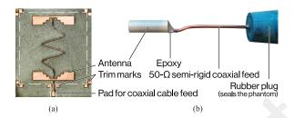
Fig. 6. Prototype manufacturing. (a) 434-MHz design patterned on a Rogers 3850HT substrate. (b) The antenna soldered to a coaxial feed, rolled, and inserted into a ceramic shell. Araldite 2012 epoxy seals the cable side. Prior to characterization, the capsule is filled with pure water and sealed with a rubber plug (not shown). For the radiation measurements, the coaxial feed is insulated from the phantom with an air-filled \$10-mm polyamide tube.
