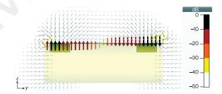
Fig. 2. Electric field generated by the proposed antennas corresponds to a conventional patch. This figure shows an **E**-field distribution example in x=0 plane of the 868-MHz design.
