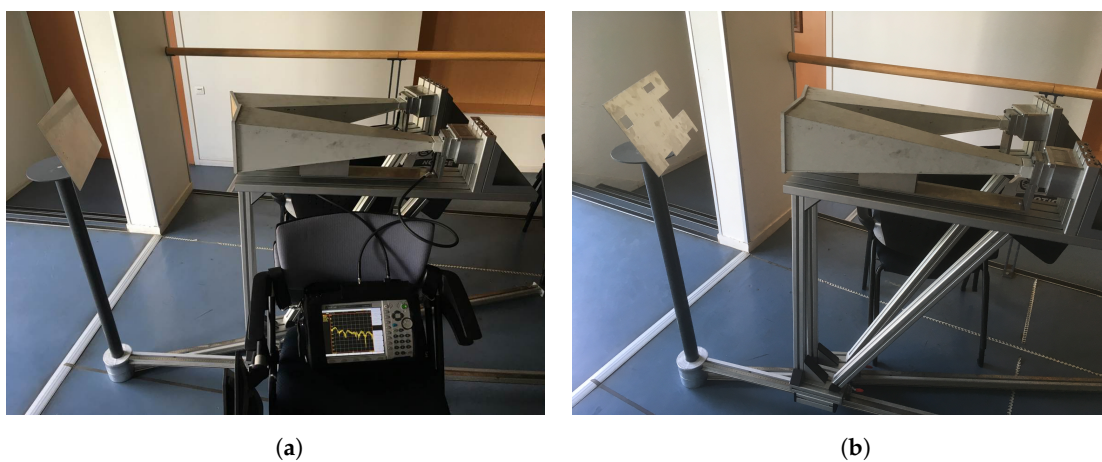
Figure 5. Measuring setup for validation for a rectangular plate (a) and a complex target (b).
