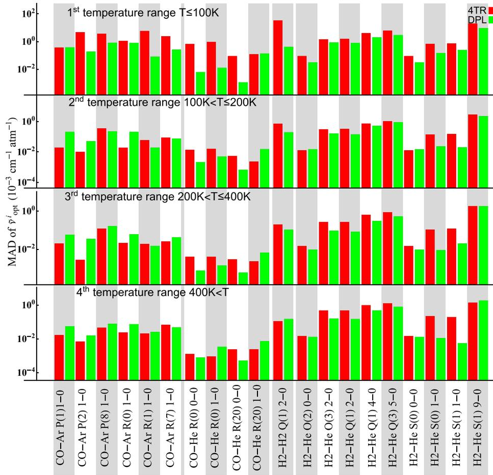
Fig. 12. The MAD for the 4TR and DPL representations of the temperature dependence of the imaginary part of the Dicke parameter,  $\tilde{\nu}_{opt}^i$  (see text for more details).
